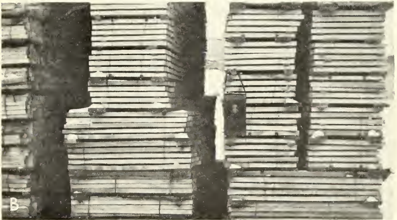
Piling of bundled dimension stock: A, Twine-bound bundles of dimension stock piled in the open; B, wire-bound and twine-bound bundles of dimension stock having stickers between courses, and also twine-bound solid bundles, all with stickers separating layers of bundles
